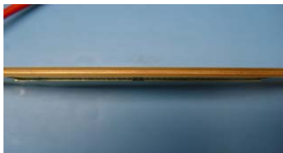
Figure 1. New 3-D CCA Assembly with Imbedded Components (Source: STI).
